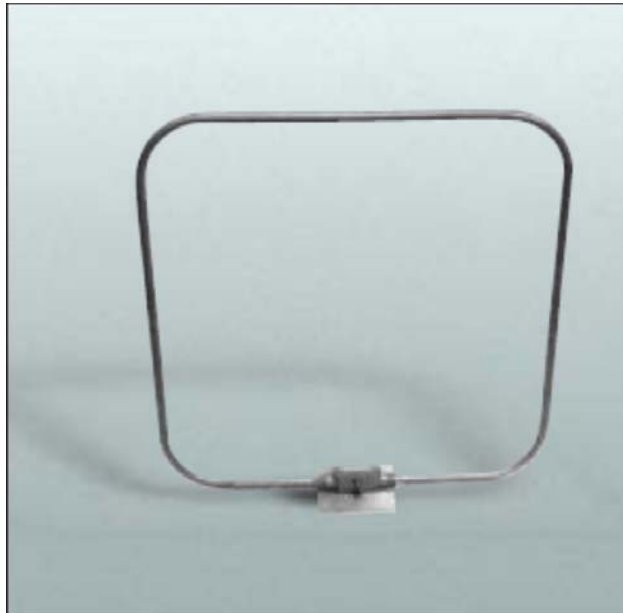
FIGURE B-4. FIXED LOOP [28.5 X 29.75-INCH, 6.31-INCH RADIUS (11 TURNS OF WIRE)]
